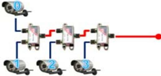
$$S_{max(4)} = 4.5\text{dB} * 3 = 13.5 \text{ dB} \quad \text{損失 } 169\text{M}$$
