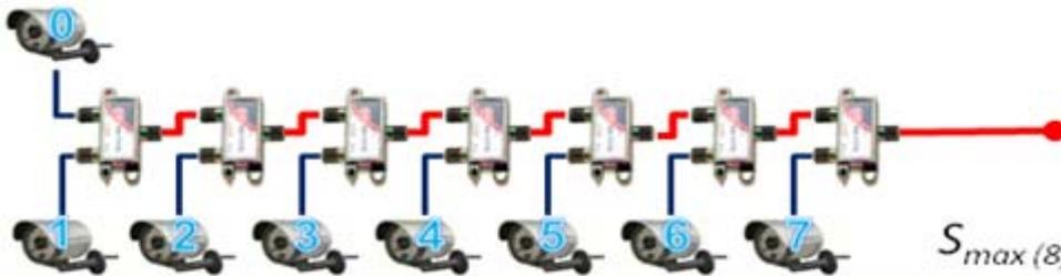
$$S_{max(8)} = 4.5\text{dB} * 7 = 31.5 \text{ dB} \quad \text{損失 } 394\text{M}$$
